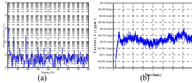
Figure 1: The performance of 62075H-30 power supply
