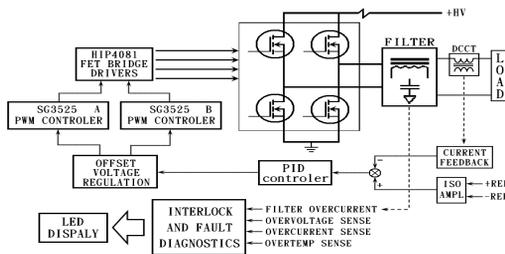
Figure 2: The structure of corrector power converter
