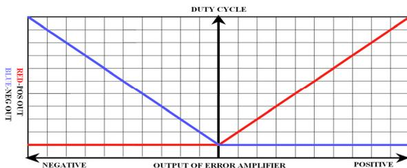
Figure 3: The relationship between the switching duty cycles and the output of error amplifier
