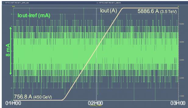
Figure 4: Ramp to 3.5 TeV for RB.A81 circuits.
