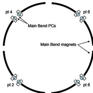
Figure 1: the 8 main dipole circuits.
