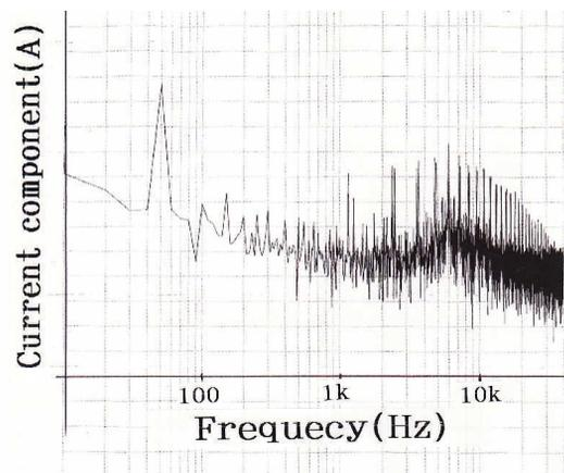
Figure 2: Fourier component of the current through the surge-suppressor in parallel with the VCB contactor.
