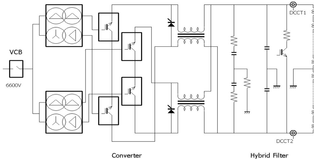
Figure 1: Principal circuit of the bending magnet power supply.
