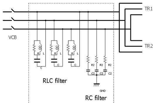
Figure 3: Filter for higher harmonic current.
