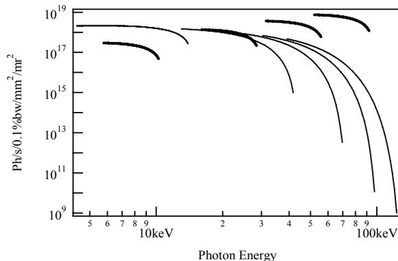
Figure 2: Tuning curves: CEBAF vs. APS; tuning curves for APS (thin black), 1st to 9th harmonics (only odd) from low to high energy; tuning curves for CEBAF (thick black), from left to right corresponding to 3.6, 6, 8.4 and 10.8 GeV (only 1st harmonic)
