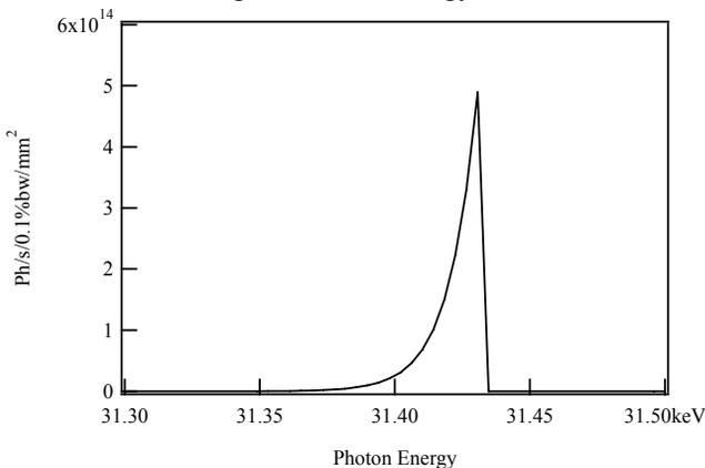
Figure 6: On-axis flux density for 8.4 GeV CEBAF.
