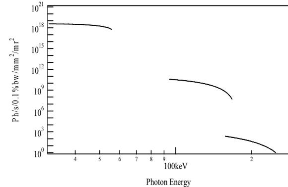
Figure 1: Tuning curves for 8.4 GeV CEBAF, 1st to 5th harmonics (only odd).
