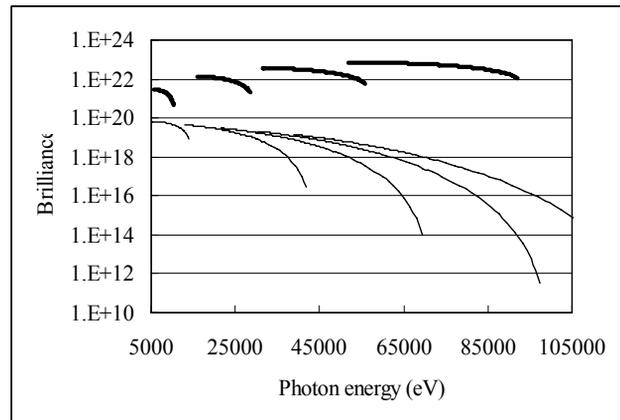
Figure 3: Peak brilliance tuning curves, 1st to 9th harmonics for APS (only odd) from low to high energy, 3.6, 6, 8.4 and 10.8 GeV (only 1st harmonic) from left to right for CEBAF, thin black for APS, thick for CEBAF.
