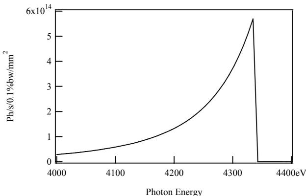
Figure 7: On-axis flux density for APS first harmonic.
