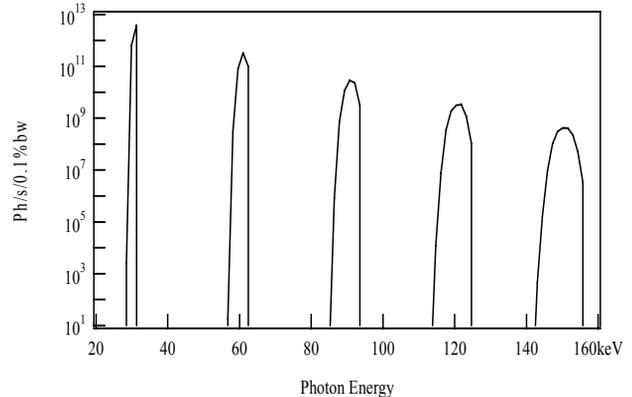
Figure 4: Spectral flux at first 5 harmonics of 8.4 GeV CEBAF.
