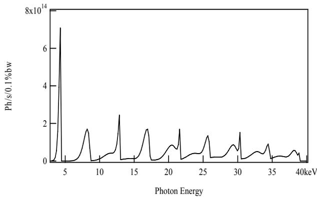
Figure 5: Spectral flux of first 9 harmonics for APS.
