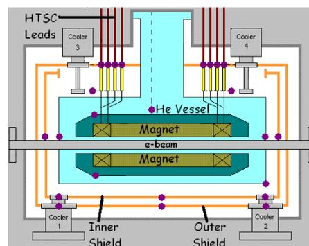
Figure 1: Illustration of Cryostat Structure.
