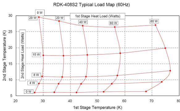
Figure 2: Typical Heat Load Map.
