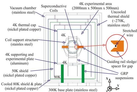
Figure 1: Drawing of the cryostat's different temperature regions and the experimental chamber with the entry for local and integral field measurement systems.
