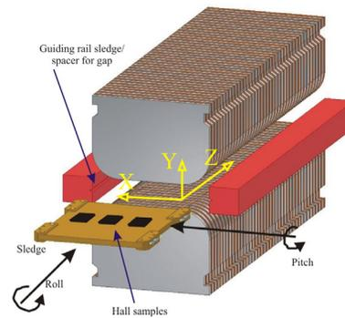
Figure 3: Sketch of the coils with the setup for local field measurements.
