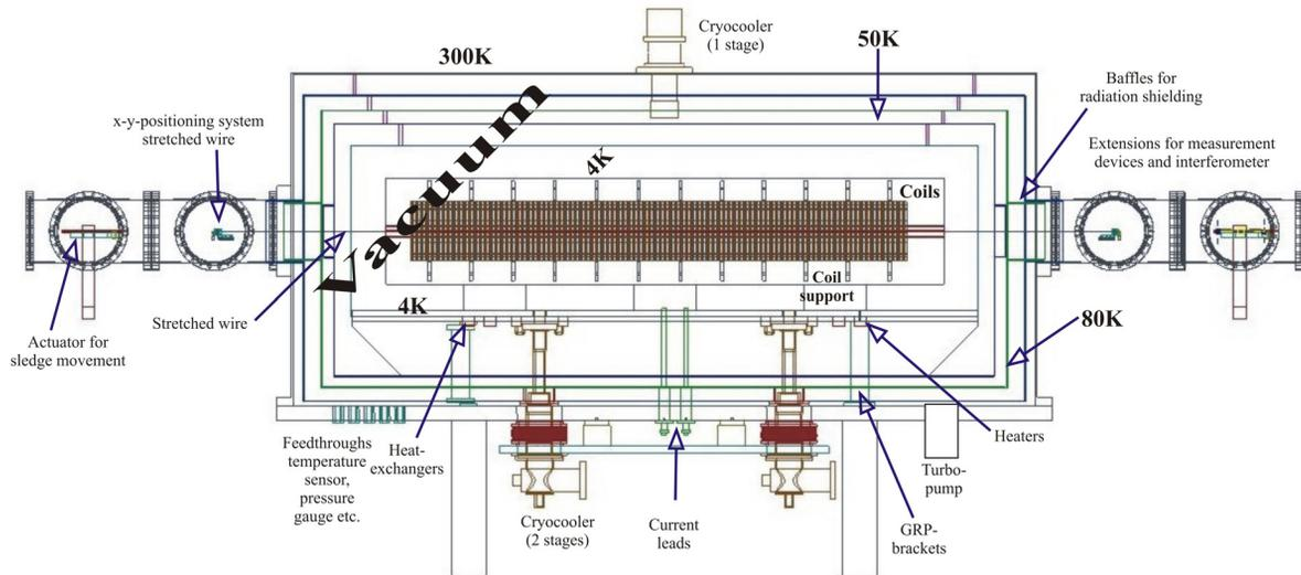
Figure 2: Side view of the cryostat (CASPER II) with the equipment for local and integral field measurements.
