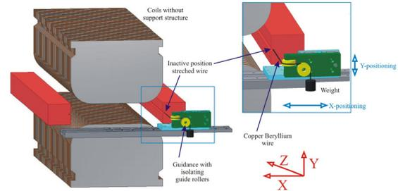
Figure 4: Drawing of the coils with stretched wire components
