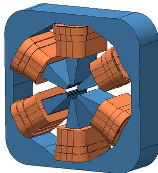
Figure 8. Multifunctional Sextupole with steering coils and skew quadrupole corrections.
