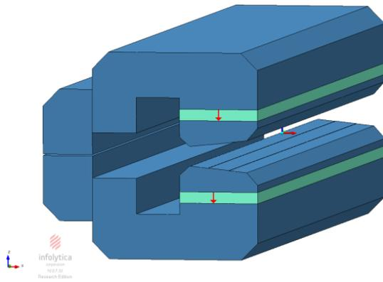
Figure 3. Mechanical design of the 0.5 Tesla dipoles.
