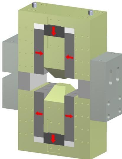
Figure 4. Mechanical design of the 2 Tesla dipole.
