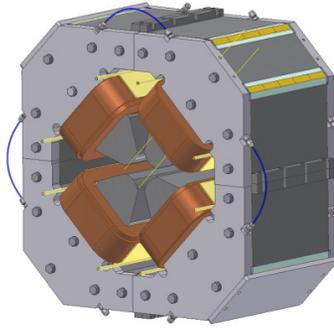
Figure 7. Mechanical design of the quadrupole.
