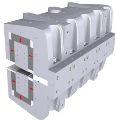
Figure 2. Mechanical design of the dipole based on ferrite – first prototype. The arrows indicate the direction of the ferrite magnetization. The main steel body was cast and the critical dimensions were machined after.
