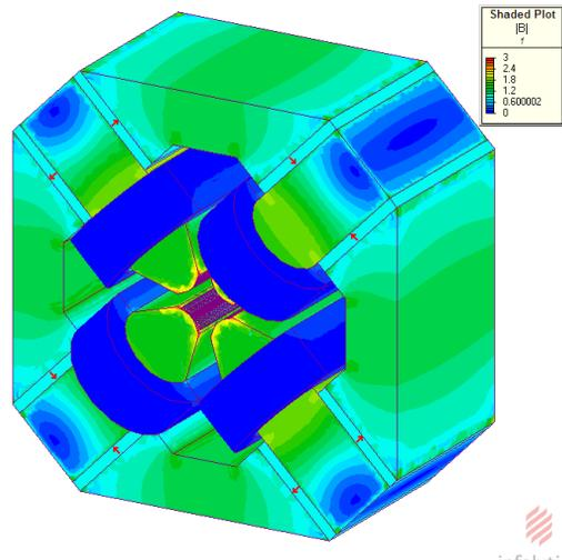
Figure 5. Magnetic simulation of the quadrupole.
