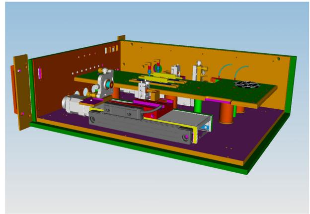
Figure 4: Schematic of the most recent BAM chassis. Visible are the two motorised delay stages and the four posts for the peltier elements underneath the aluminium plate on which both EOMs are installed.
