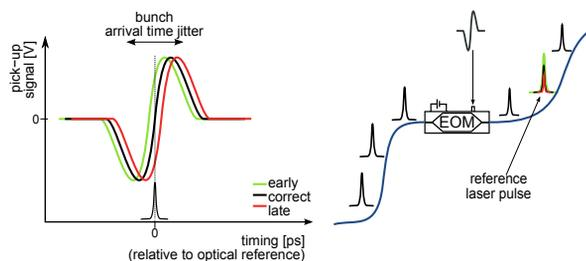
Figure 2: Schematic of the BAM detection scheme utilising electro-optical modulation.
