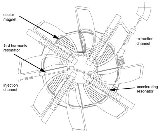
Figure 2: Schematic top view of the PSI Ring cyclotron.
