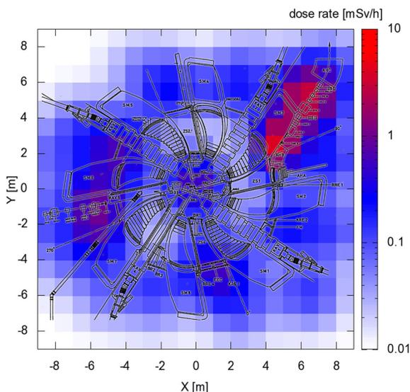
Figure 6: Map of residual dose rates in the Ring cyclotron. The map is interpolated from ~30 data points.
