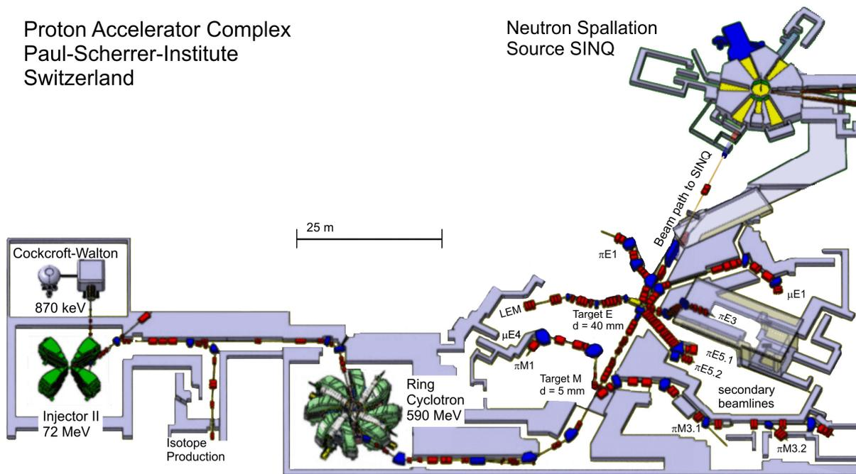
Figure 1: Overview of the PSI high intensity accelerator complex.
