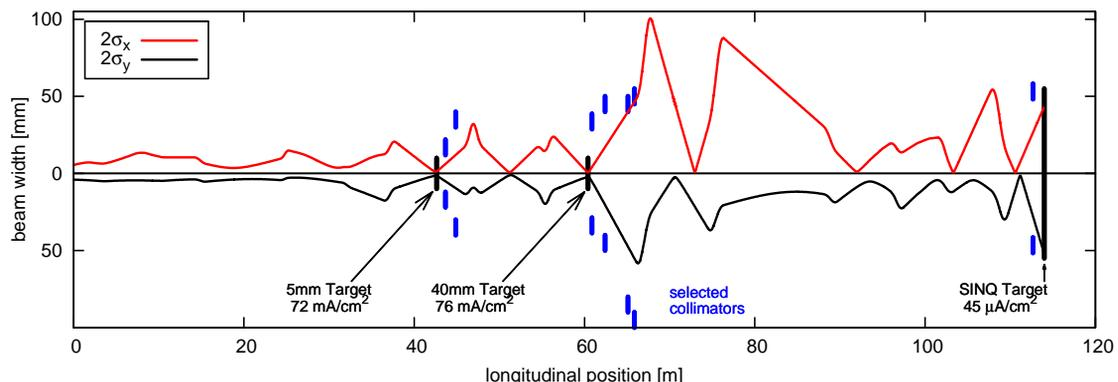
Figure 5: Horizontal and vertical beam envelopes in the transfer line from Ring cyclotron to SINQ. The two meson production targets and the SINQ spallation target are indicated with current densities. Selected collimators are shown.
