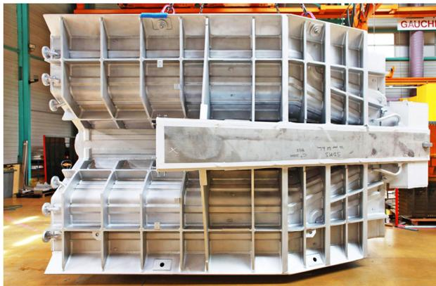
Figure 8: New 50 MHz accelerating resonator for the Injector II cyclotron in the PSI HIPA facility.
