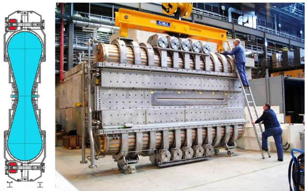
Figure 7: Cross section (left) and photograph of the 50 MHz accelerating resonator of the Ring cyclotron.
