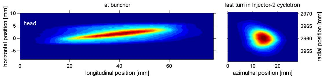
Figure 4: Particle density for a current of 2.2 mA at 72 MeV, measured at the exit of the PSI Injector II cyclotron (right) and after an additional drift length of ~20 m. The strong blowup in a comparably short drift space demonstrates the strong focusing effect of the circular beam regime within the Injector II cyclotron.
