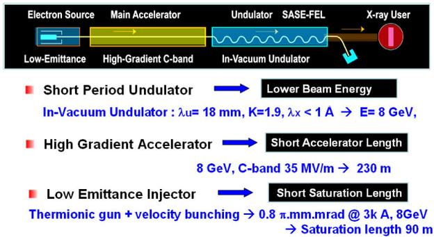
Figure 2: SCSS concept makes FEL machine compact.
