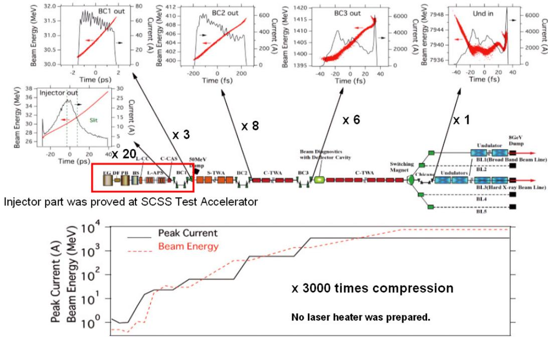
Figure 4: Machine configuration and beam parameters in 8 GeV XFEL/SPring-8.
