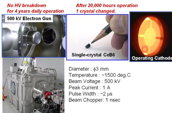
Figure 3: CeB<sub>6</sub> single crystal thermionic cathode for low emittance electron source.
