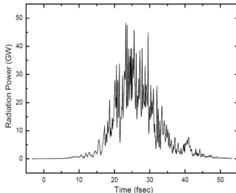
Figure 7: Simulated FEL output power at 1 Å wavelength.
