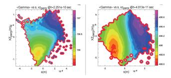
Figure 3: False color image showing  $\bar{\gamma}(s,r_\perp)$  at the simulation end for both the 100-MeV case of Figs. 1&2 (left plot) and a much shorter pulse ( $\sigma_z=4.5\,\mu\mathrm{m}$  at 250-MeV traversing a 0.5-m long dipole with 26.7 m radius of curvature. Negative (positive) values of  $r_\perp$  correspond to particles whose transverse position (presuming laminar flow) was on the outer (inner) portion of the arc.
