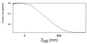
Figure 2: Mean energy loss in units of  $mc^2$  versus lab position in z for the 500 A, 150-fs duration pulse of Fig. 1. The 0.5-m long dipole magnet begins at z=0 m.
