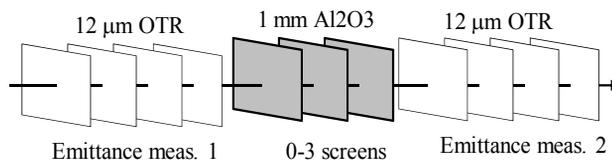
Figure 1: Schematic of the measurement using a total of 11 screens (2×4 for emittance measurement, and 0-3 for scattering the beam).
