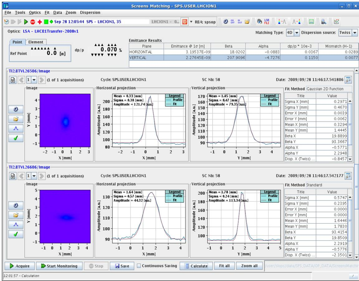
Figure 2: Image from the ScreenMatching application used to measure the emittances in TI 2 with Pb<sup>82+</sup> ions. The dp can either be specified or fitted from the data.
