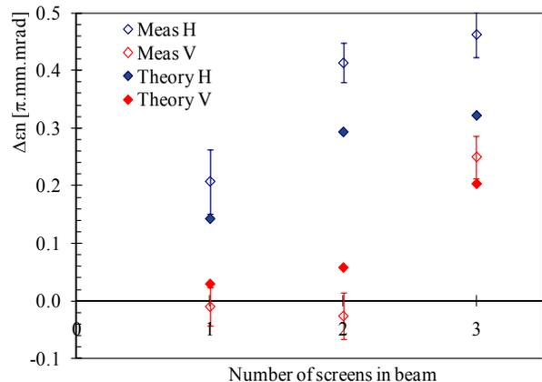
Figure 3: Normalised emittance growth of 177 GeV/u Pb<sup>82+</sup> ions from 1.4 mm thick alumina screens in TI 2, compared to expectation from simple theory.
