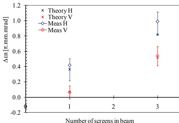
Figure 5: Normalised emittance growth of 450 GeV p+ ions from 1.4 mm thick alumina screens in TI 2, and expectation from simple theory.
