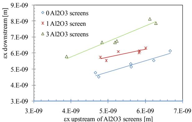
Figure 4: Correlation plot showing how the horizontal Pb<sup>82+</sup> emittance measured downstream of the scatterers depends on the emittance upstream, over a number of measurement points.
