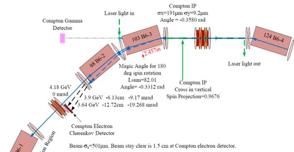
Figure 1: Layout of the Compton polarimeter.
