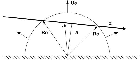
Figure 3: Scheme of the electron bunch motion through Mg gas cloud
