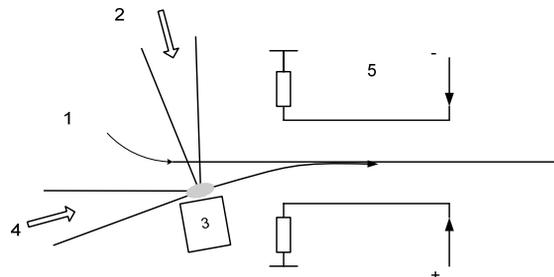
Figure 1: Layout of injection in a cyclic accelerator using LWFA. 1 – closed orbit, 2 – evaporating light, 3 – Mg target, 4 – accelerating light, 5 – fast kicker.
