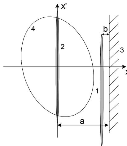
Figure 2: Scheme of injection in the phase plane. 1 - injected beam, 2 - injected beam after the kick, 3 - the wall, 4 – the acceptance ellipse.
