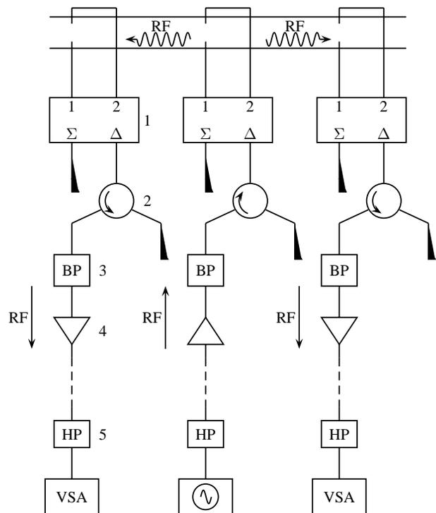
Figure 4: Schematic overview of the experimental setup containing hybrids (1), circulators (2), band passes (3), amplifiers (4) and high passes (5).
