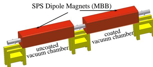
Figure 1: Schematic overview of the transmission sections. The left dipole has the uncoated, the right dipole the coated vacuum chamber.
