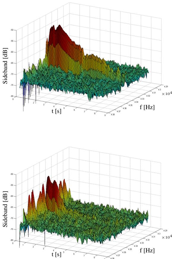
Figure 5: Phase modulation sideband versus time and frequency in case of the uncoated (upper graph) and coated (lower graph) vacuum chamber. The signal in the coated section vanishes shortly after injection, whereas in the uncoated section the signal remains well above the noise floor. The large signal in the beginning corresponds to the injection of the beam where the used electronics are driven into saturation. The valid range for evaluation starts about 3 s after injection.
