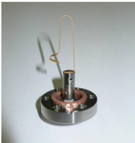
Figure 3: Picture of a coupling loop used for the injection and pickup of the microwave signal.
