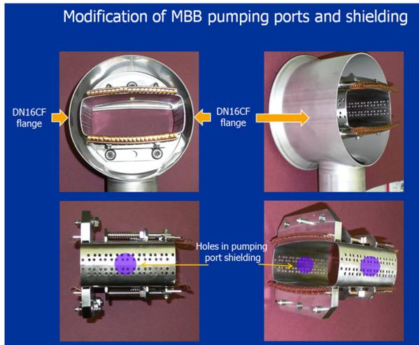
Figure 2: Principle of the SPS MBB pumping port and shielding modifications necessary for the integration of the microwave transmission coupling loops.
