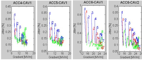
Figure 2: Jitter along the probe signal flat top as a function of cavity gradient. The numbers refer to the data set and the colors refer to the detuning as in Fig. 1.
