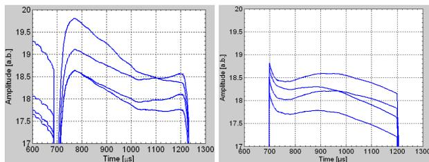
Figure 10: 2<sup>nd</sup> input rf flat top waveforms. Left: 3MHz/3nC beam with 1600 bunches and piezos off; Right: 3MHz/3nC beam with 1500 bunches and piezos on.
