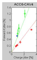
Figure 11: 2<sup>nd</sup> input rf flat top jitter as a function of bunch charge jitter and the expected slopes ( $1/2$  for the green solid line,  $1/4$  for the red). The colors are as in Fig. 9.
