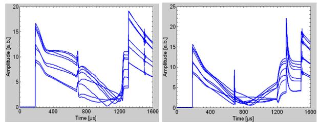
Figure 13: Reflected rf waveforms for cavities in ACC6. Left: 3MHz/3nC beam with 1600 bunches and piezos off; Right: 3MHz/3nC beam with 1500 bunches and piezos on.
