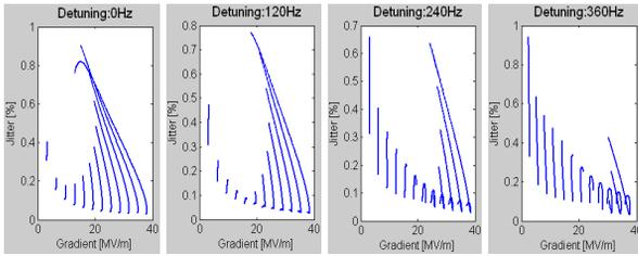
Figure 3: Analytical estimates of the probe signal flat top jitter versus cavity gradient for the specified detuning.
