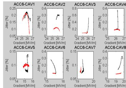
Figure 8: Probe signal flat top jitter with piezos on and off for nominal detuning. Red: piezos off; black: piezos on.
