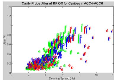
Figure 7: Probe signal jitter at the end of the rf pulse versus detuning jitter for all cavities/detunings.
