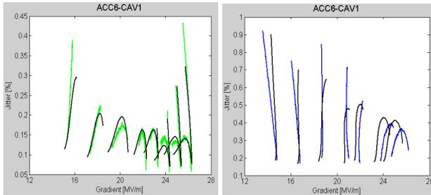
Figure 5: Comparison between data and simulated probe signal jitter for different detuning. Green: nominal-100Hz; blue: nominal+100Hz; black: simulation.
