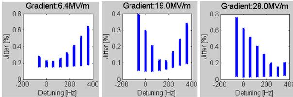
Figure 4: Analytical estimates of the probe signal flat top jitter versus detuning for the specified cavity gradient.
