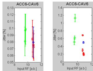
Figure 9: 1<sup>st</sup> (left) and 2<sup>nd</sup> (right) input rf flat top jitter as a function of rf amplitude. Red: 1MHz/3nC beam with piezos off; Blue: 3MHz/3nC beam with piezos off; Green: 3MHz/3nC beam with piezos on.
