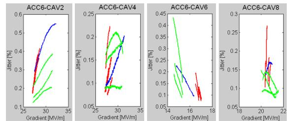
Figure 12: Probe flat top jitter as a function of gradient. The colors are as in Fig. 9.
