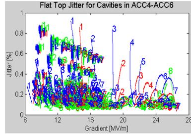
Figure 6: Probe signal jitter for all cavities/detunings.
