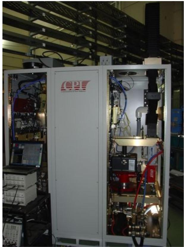
Figure 5: CPI 90 kW Power amplifier.
