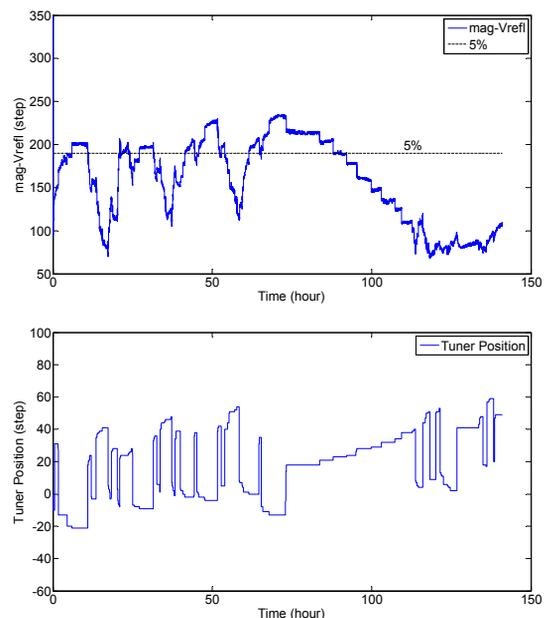
Figure 3: Amplitude of the reflected voltage (above) and tuner position (below) measured during a period of 140 hours
