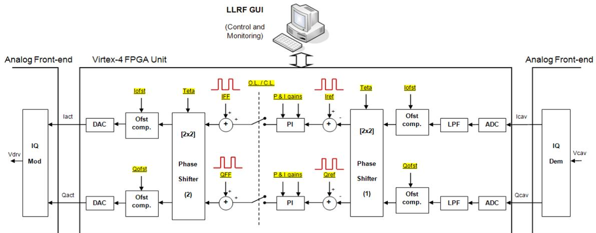
Figure 4: Simplified schematics of the FPGA program for amplitude and phase regulation; the parameters which are marked as underscore are set from the control computer.
