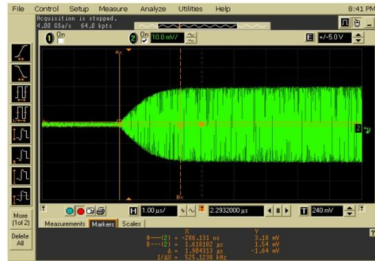
Figure 2: Measured cavity field in pulsed mode
