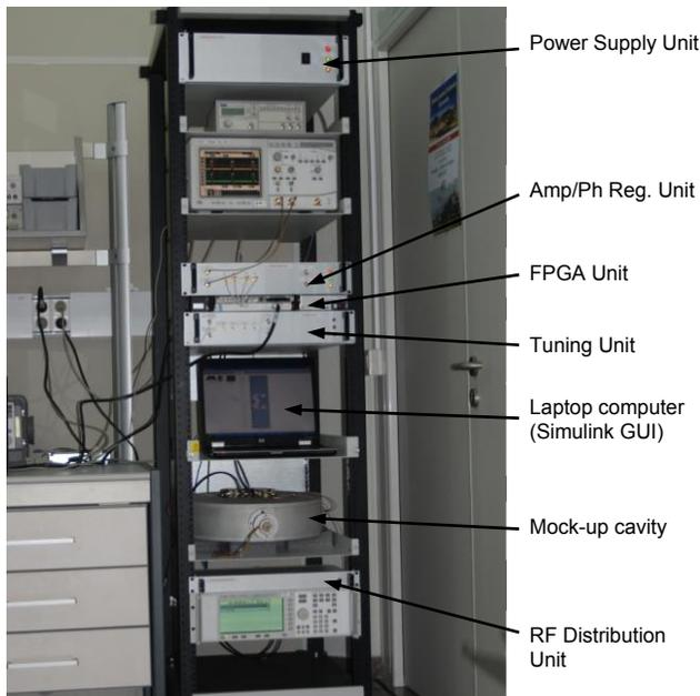
Figure 1: Picture of the LLRF test setup
