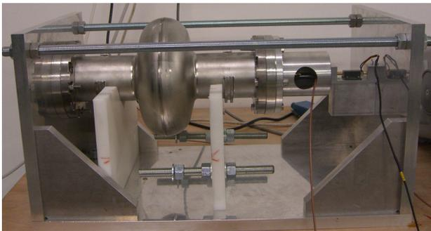
Figure 6: The cavity and piezo-actuators.
