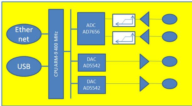
Figure 2: Block diagram of the digital section.
