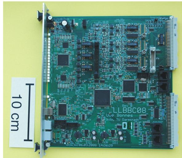
Figure 4: Picture of the S-DALINAC FPGA board.
