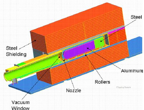
Figure 1: Cross sectional view of the new off-momentum beam stop and vacuum assembly.
