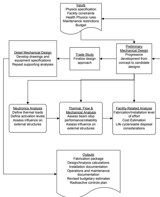
Figure 5: Design methodology flow chart.
