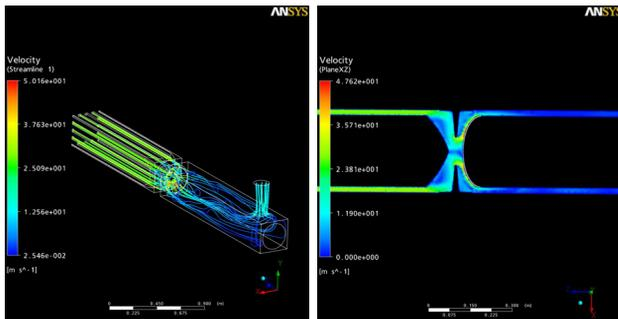
Figure 3: CFD simulation results for beam stop assembly
