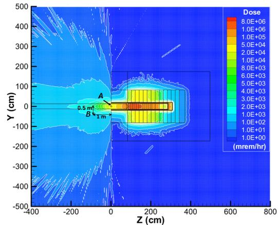
Figure 4: Aluminum beam stop activation at Na-22 saturation levels (16 years of operation at 10 kW) followed by 1 month decay
