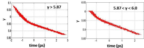
Figure 3: Longitudinal phase space of the bunch head at position 43.5 cm away from the gun exit.
