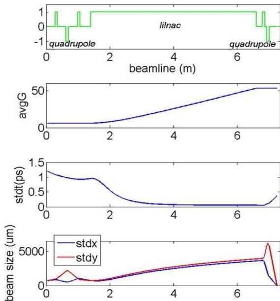
Figure 4: The evolution of beam characteristics from the exit of alpha magnet to the interaction point.
