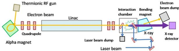
Figure 1: The layout of the NSRRC ultrashort electron beamline for ICS experiment.
