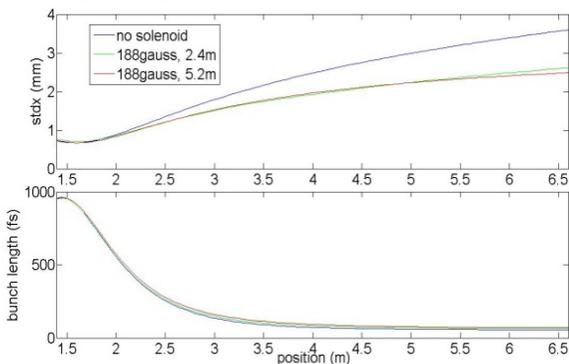
Figure 5: The different evolution through linac by applying the solenoid.
