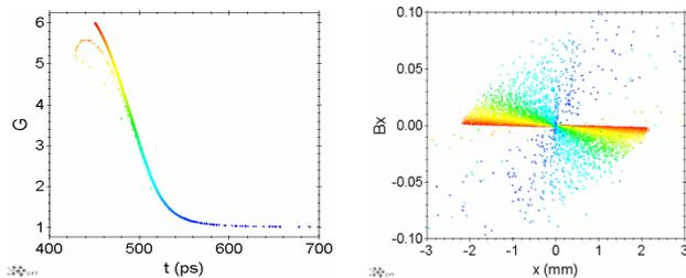
Figure 2: The longitudinal and transverse phase spaces of electron beam at the gun exit.
