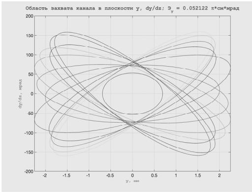
Figure 3: Acceptances in the plane (y, dy/dz) without radial matching section.
