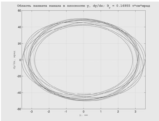
Figure 5: Acceptances in the plane (y, dy/dz) with radial matching section.
