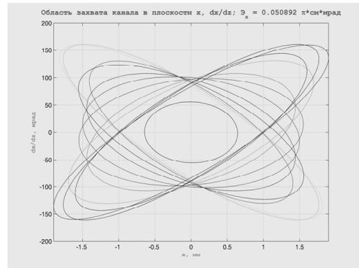
Figure 2: Acceptances in the plane  $(x, dx/dz)$  without radial matching section.
