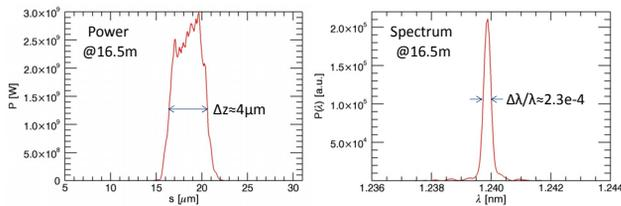
Fig. 3: FEL-3 pulse profile (left) and spectrum (right).
