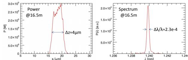
Fig. 3: FEL-3 pulse profile (left) and spectrum (right).
