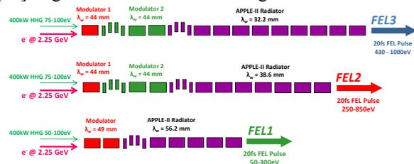
Fig. 2: Schematic of the revised harmonic cascade FEL scheme; blocks represent undulator module 2.5 m long.
