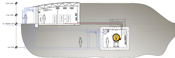
Fig. 5: Linac tunnel and RF services building
