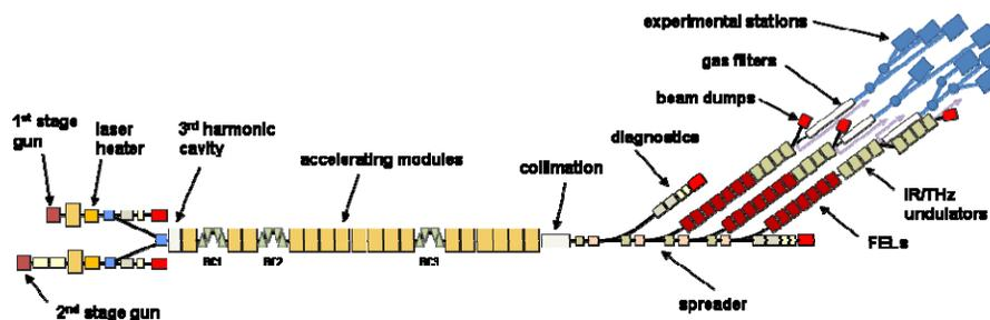
Fig. 1: Schematic layout of the NLS facility
