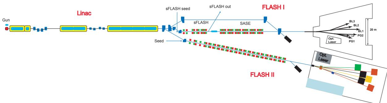
Figure 2: Schematic layout of the FLASH facility. The electron gun is on the left, the experimental hall on the right. Behind the last accelerating module, the beam is switched between FLASH I, which is the present undulator line, and FLASH II, which is the upgrade. Behind the extraction point, space is reserved for an additional laser system for seeding.
