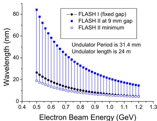
Figure 3: Tunability range of FLASH II for a given energy determined by FLASH I users.
