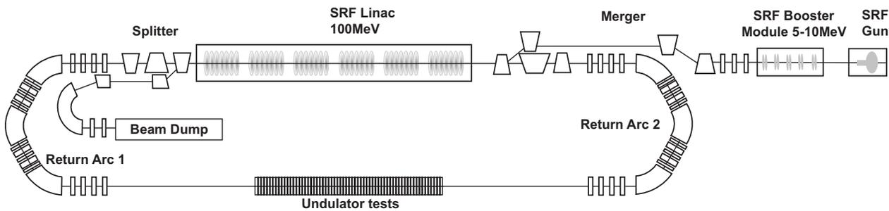
Figure 1: BERLinPro: schematics of the ERL prototype.
