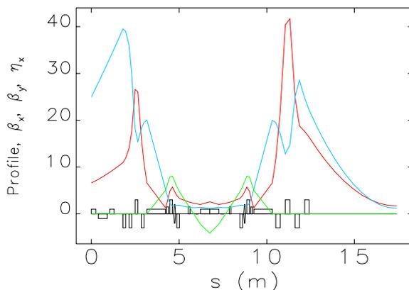
Figure 2: Magnet lattice and Twiss-parameter for the first half of the BERLinPro recirculator in "Normal Operation" ( $R_{56} = 0$  m). red:  $\beta_x$ , blue:  $\beta_y$ , green:  $\eta_x \cdot 10$ .
