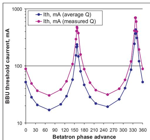
Figure 4: *BERLinPro*: BBU threshold currents vs recirculator phase advance for two HOM sets.
