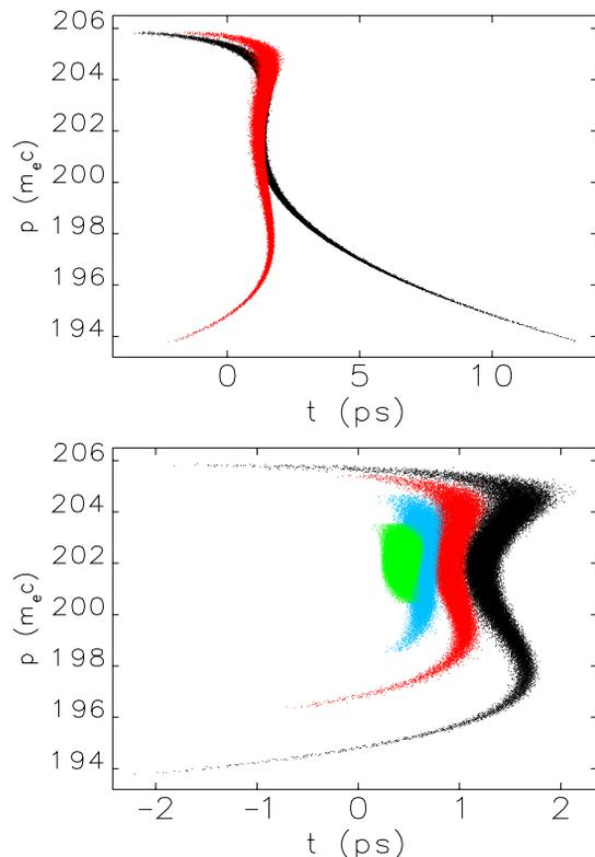
Figure 3: Short pulse mode: top) long. phase space without (black) and with (red) multipoles, ( $\sigma_{l,i} = 2.0$  mm); bottom) long. phase space for bunches of minimized length starting with various initial pulse lengths out of the linac:  $\sigma_{l,i} = 2.0$  (black) / 1.5 (red) / 1.0 (blue) / 0.5 (green) mm  $\rightarrow \sigma_{l,f} = 73/34/21/20 \mu\text{m}$ .
