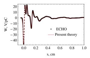
Figure 3: Wakepotential of a  $\sigma_z = 100 \ \mu m$  bunch.
