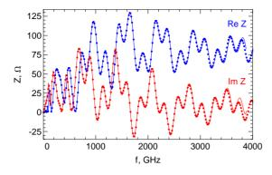
Figure 2: Collimator impedance: present theory is shown with solid line, the results of simulations with ECHO are shown with dots.
