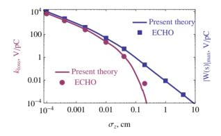
Figure 4: Loss factor and maximum of the wakepotential.
