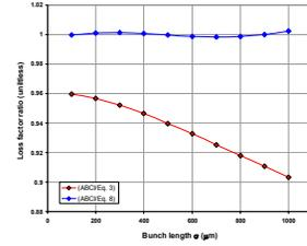
Figure 7: Comparison of loss factor ABCI with respect to those calculated using Eq. 3 and Eq. 8.
