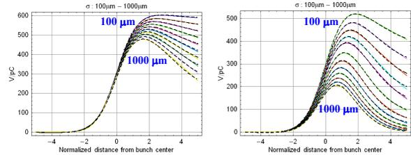
Figure10: transverse wakes calculated by the new ABCI model (black dashed) vs. ABCI (coloured) for step-out transition case (left) and taper-out transition (right).
