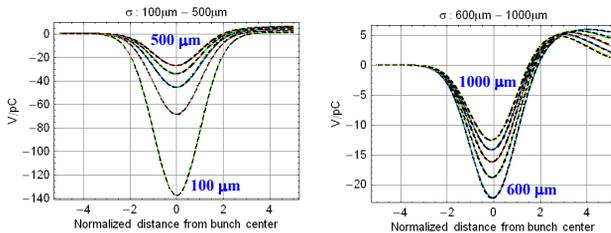
Figure 9: Longitudinal wakes calculated by the new ABCI model (black dashed) vs. ABCI (coloured) for taper case.
