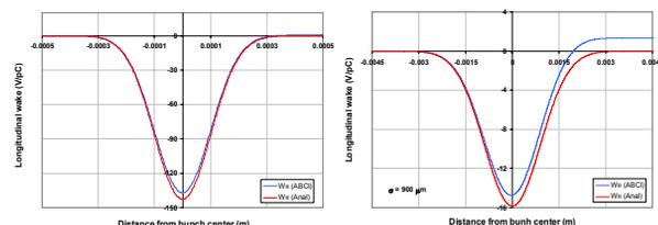
Figure 3: Numerical and analytical longitudinal wake potentials of the step-out transition at 100  $\mu\text{m}$  and 900  $\mu\text{m}$  rms bunch lengths
