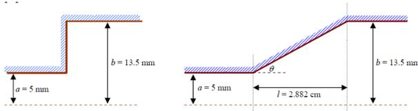
Figure 1: Lay out of the step-out and tapered-out transitions of X-band structure to the beam tubes.
