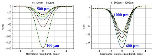
Figure 6: Longitudinal wakes calculated by the new ABCI model (black dashed) vs. ABCI (coloured) for step case.
