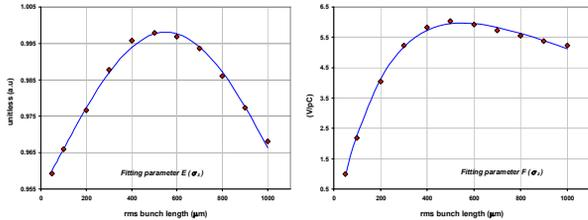
Figure 8: Fitting parameters  $E(\sigma_z)$  and  $F(\sigma_z)$  as a function of bunch length.
