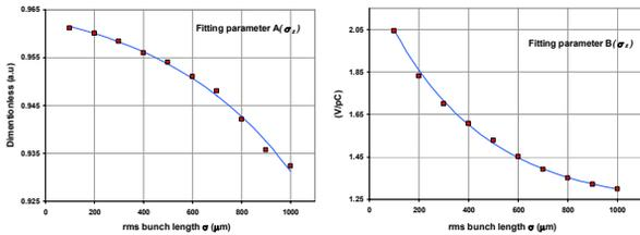
Figure 5: Fitting parameters  $A(\sigma_z)$  and  $B(\sigma_z)$  as a function of bunch length.
