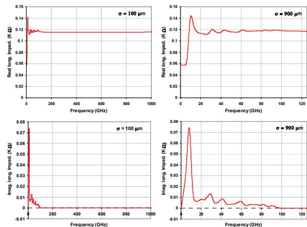
Figure 2: Real and imaginary impedances of the step-out transition at 100  $\mu\text{m}$  and 900  $\mu\text{m}$  rms bunch lengths
