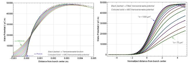
Figure 4: Left: transverse wake potentials (solid lines) and the transverse wake function (dashed line) of the X-band structure. Right: Numerical (solid lines) and analytical (dashed lines) transverse wake potentials normalized to rms  $\sigma$  of the electron bunch
