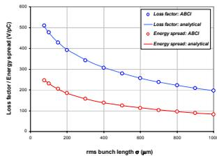
Figure 3: Loss factor (blue) and energy spread (red) obtained numerically by ABCI (circles) and those obtained analytically (lines) of the X-band structure.
