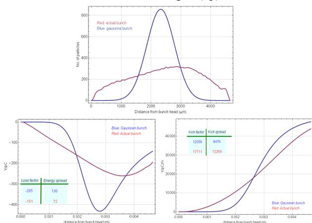
Figure 6: Longitudinal and transverse wake potentials of 4.65 mm electron bunch of Gaussian distribution (blue) and actual distribution (red). Both distributions are normalized to 1 pC.
