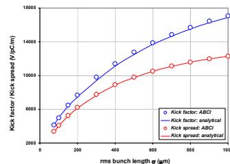
Figure 5: Kick factor (blue) and kick spread (red) obtained numerically by ABCI (circles) and those obtained analytically (lines) of the X-band structure.
