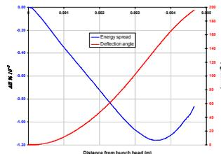
Figure 7: Induced energy spread and deflection angle due to wake potentials along the 4.65 mm electron bunch at FERMI@ELETTRA FEL.
