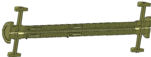
Figure 1: Cut view of X-band structure showing the mode launchers and wakefield monitors.
