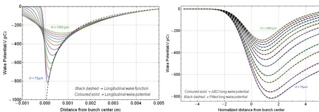
Figure 2: Left: longitudinal wake potentials (solid lines) and the longitudinal wake function (dashed line) of the X-band structure. Right: Numerical (solid lines) and analytical (dashed lines) longitudinal wake potentials normalized to rms  $\sigma$  of the electron bunch
