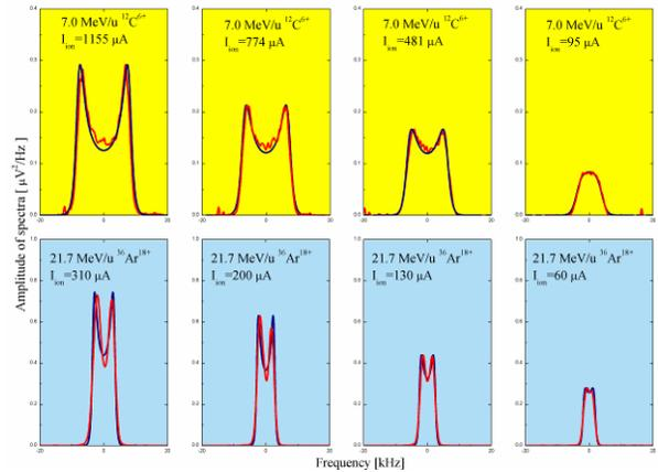
Figure 2: Schottky spectra of measured and calculated for various ion beam currents. Blue line shows the measurement data and red line is simulation result.
