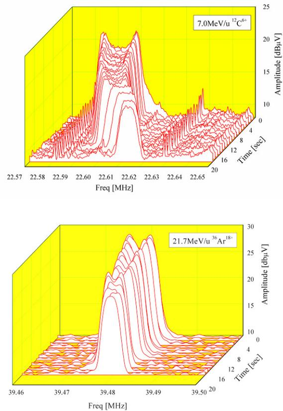
Figure 1: sequence of Schottky spectra for  $^{12}\text{C}^{6+}$  and  $^{36}\text{Ar}^{18+}$  at the 100<sup>th</sup> harmonic of the revolution frequency show a double-peak phenomenon at high beam density.
