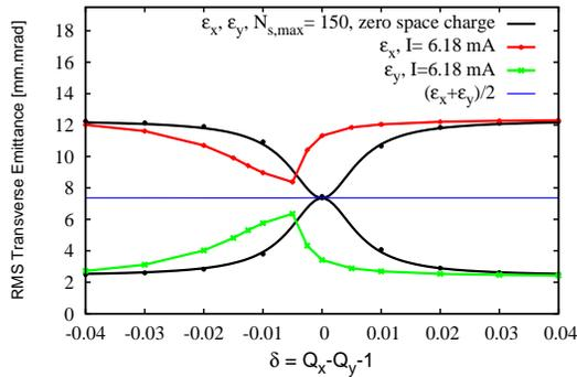
Figure 3: Emittance exchange simulation using PARMTRA. The incoherent tunes shift are  $\Delta Q_x = -0.02$ ,  $\Delta Q_y = -0.11$  with applied skew quadrupole strength,  $k_{sq} = 5 \times 10^{-3} \text{ m}^{-1}$ .
