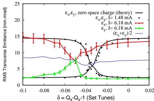
Figure 4: Emittance exchange measurement (06Aug2009) using RGM due to random skew quadrupole components. The incoherent tune shifts for the high intensity beams are  $\Delta Q_x = -0.01$ ,  $\Delta Q_y = -0.10$ .
