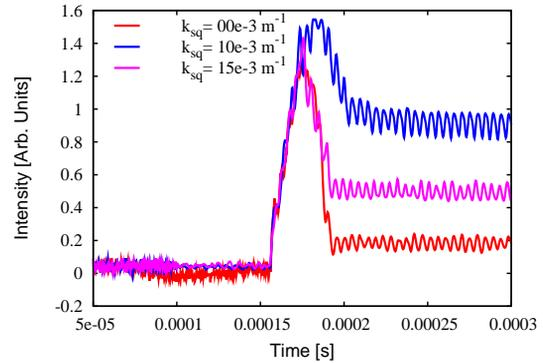
Figure 5: Current intensity in SIS18 versus time measured during multi turn injection with fast current transformer.
