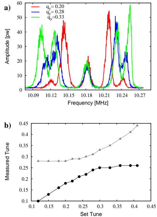
Figure 1: a) Schottky vertical spectrum measurement at SIS18 during static scan of the vertical set tune. b) the coupled tunes against the fractional vertical set tune.
