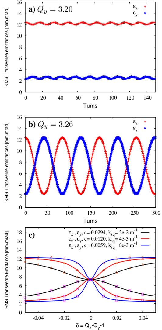
Figure 2: Transverse RMS emittance exchange simulation for zero space charge in a constant focusing lattice.
