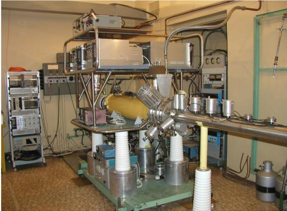
Figure 1: Electron String Ion Source Krion-2.
