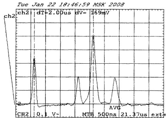
Figure 3: Spectrum of charged ions ( $H^+$ ,  $C^{5+}$ ,  $C^{4+}$ ,  $C^{3+}$  pics).
