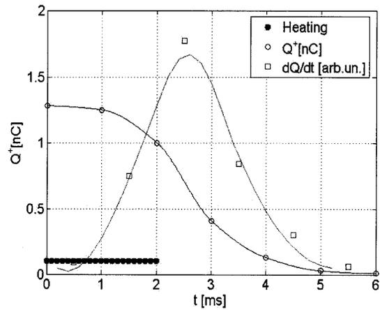
Figure 2: Total ion charge and its derivative versus start of heating and start of ion accumulation at 2 ms duration of heating pulse and ion accumulation-ionization time 10 ms.
