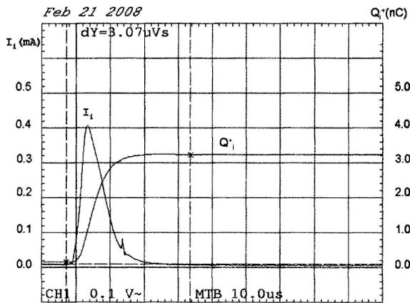
Figure 4: Total ion charge per methane injection pulse.
