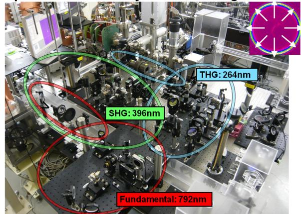
Figure 4: Optical set-up to generate a radial polarized hollow laser beam @263, 396, 790 nm: To generate a femtosecond laser pulse at the cathode, a negative-chirped laser pulse is generated at the laser source with an AO-modulator (DAZZLER HR-800, FASTLITE) to be compensated with the material dispersions.
