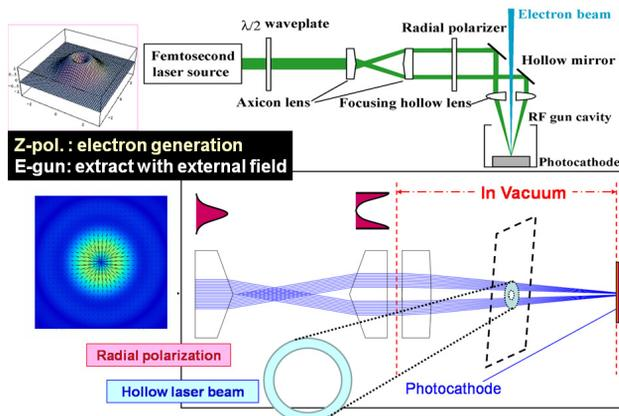
Figure 2: Schematic drawing of a Z-polarization gun with hollow laser beam incidence optics.
