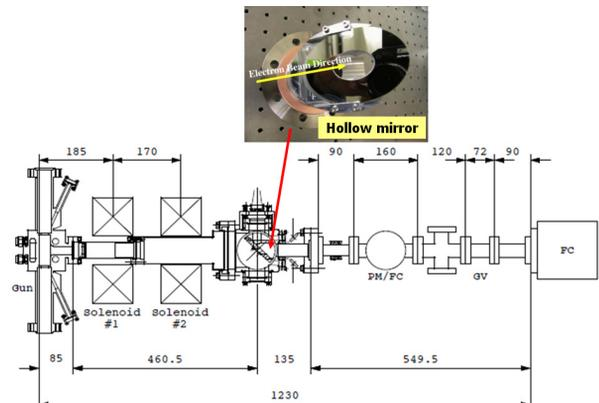
Figure 8: Experimental set-up for Z-polarization RF gun with hollow laser beam incidence optics.
