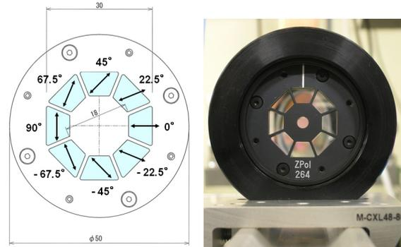
Figure 3: 8-divided waveplate (designed for femtosecond; optical-contact) manufactured by Nanophoton Corporation for a hollow beam @ 264 nm: the photo of 8-divided waveplate for a hollow beam (in right) and the direction arrangement of optical axes in each segment (in left) are shown.
