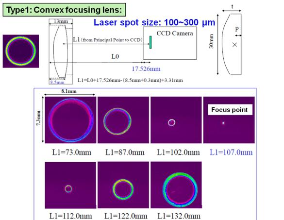
Figure 6: Focus test with a convex lens with a hollow beam.
