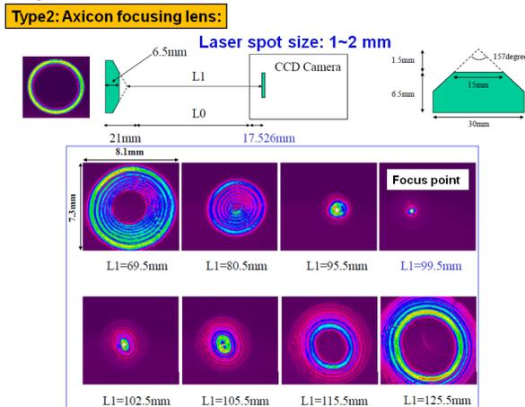
Figure 7: Focus test with an axicon lens with a hollow beam.
