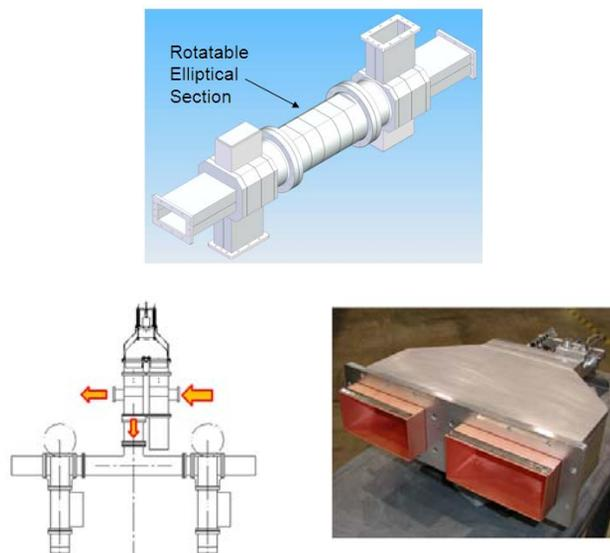
Figure 6. Top: Variable Tap-Off power splitter, bottom: system with same functionality that employs U-bend phase shifters (prototype on right).
