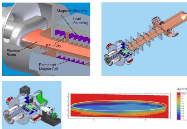
Figure 3. Top: layout of the original SBK, bottom: Beam Tester and measured beam current density after the gun.
