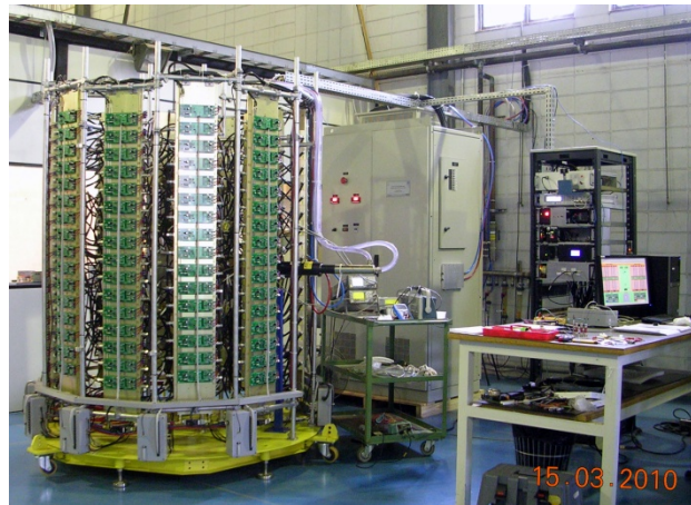
Figure 1: 476 MHz Solid State Amplifier tower being commissioned at the RF test area at the LNLS.
