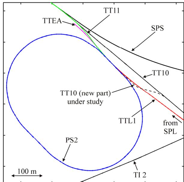
Figure 1: Layout of PS2 and its transfer lines. The dashed line represents the proposed location for the new TT10 transfer line which is currently under study.
