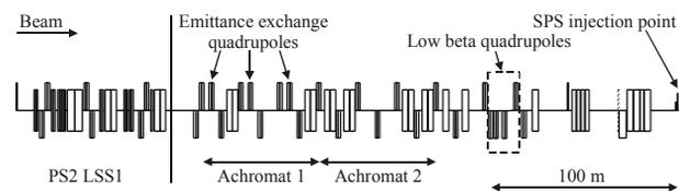
Figure 4: Layout of the TT11 transfer line.
