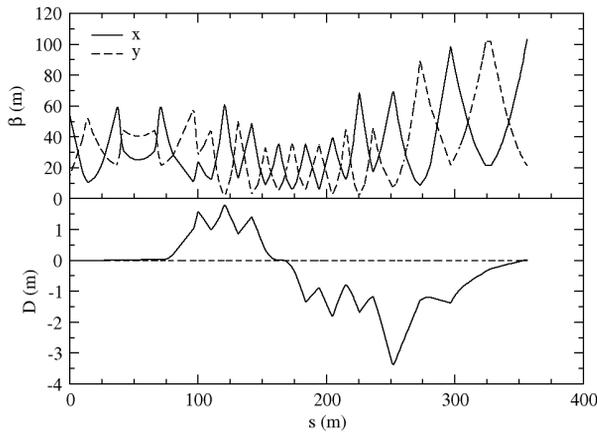
Figure 5: Simulated beta and dispersion functions along the TT11 transfer line for an LHC type proton beam.
