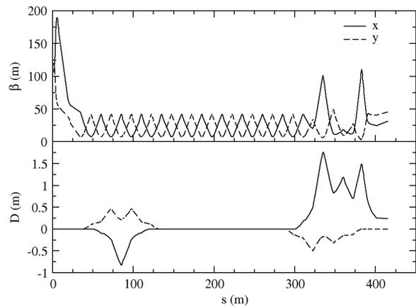
Figure 3: Simulated beta and dispersion functions along the TTL1 transfer line.
