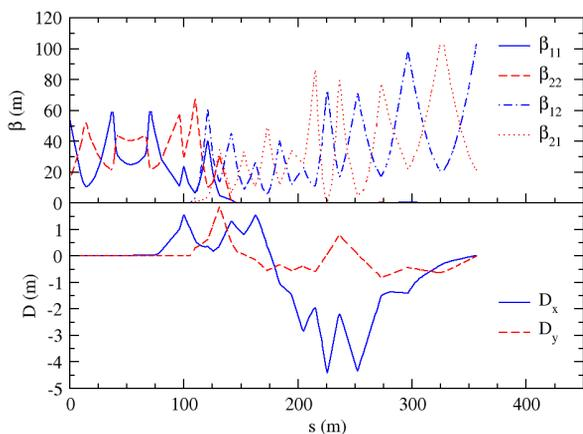
Figure 7: Simulated Ripken optics parameters and dispersion functions along the TT11 transfer line for a CNGS type beam with the skew quadrupoles powered.
