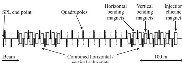
Figure 2: Layout of the TTL1 transfer line.
