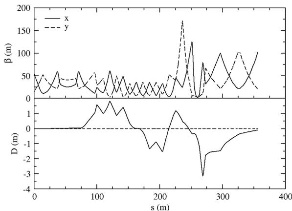
Figure 6: Simulated beta and dispersion functions along the TT11 transfer line for an LHC type lead ion beam.
