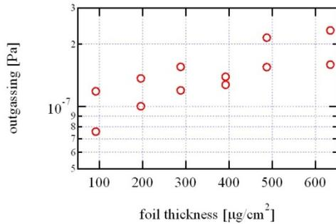
Figure 7: Pressure increments of the vacuum right after the first beam irradiation and 40 minutes later as a function of the foil thickness measured with beam.
