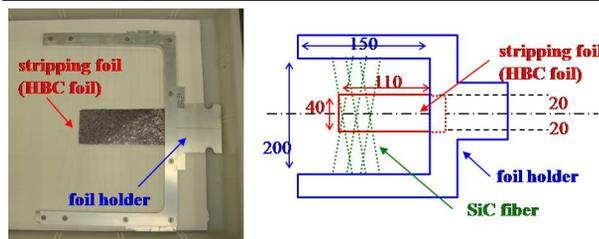
Figure 1: Schematic diagram of the operational foil mounting on the C-shaped holder.
