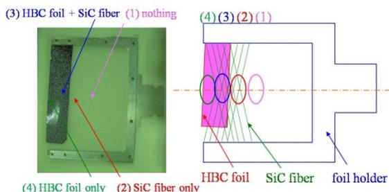
Figure 2: Schematic diagram of the extra-mounting foil to examine the effect of SiC fibers. This foil has following four areas: (1) nothing, (2) SiC fibers only, (3) HBC foil + SiC fibers, and (4) HBC foil only.
