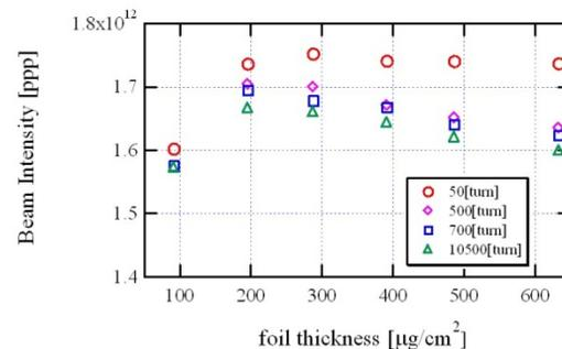
Figure 6: Typical results of the charge exchange efficiency and beam loss caused by the foil scattering as a function of the foil thickness.
