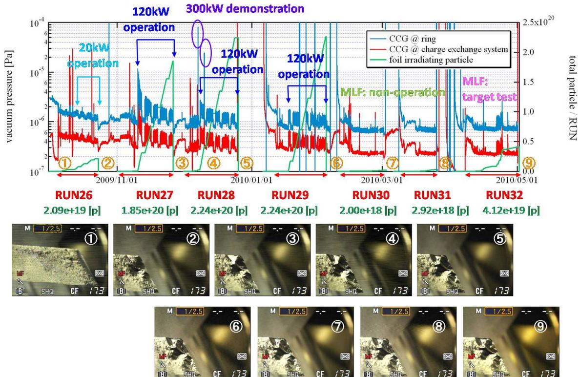
Figure 8: Trends of outgassing from the foil and the deformations on the foils during the beam irradiation. The upper graph plots the vacuum pressure measured by the CCG around the stripping foil and the total irradiated particle every run cycle. The lower photos show the deformations of the HBC foils during the beam irradiation.
