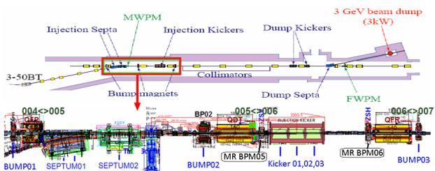
Figure 1: The layout of MR Injection section.
