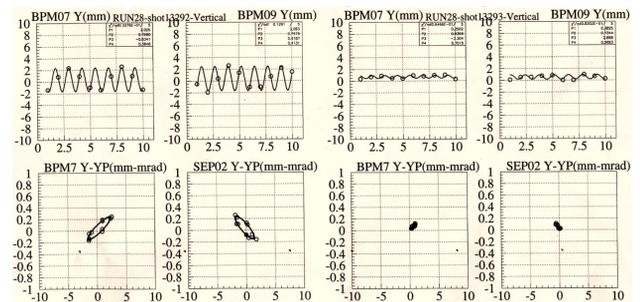
Figure 7: MR injection tuning after building bump orbit.
