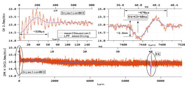
Figure 5: Analysis of MR horizontal beam position data at IPM (1<sup>st</sup> black circle: at injection timing; 2<sup>nd</sup> black circle: at latter fired timing of the injection septum 02).
