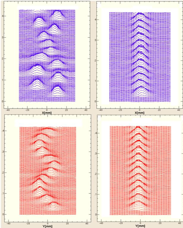
Figure 9: Horizontal (upper) and vertical (lower) beam profile mountain views for the first twelve turns measured with IPM. (Left: before injection orbit correction; Right: after injection orbit correction).
