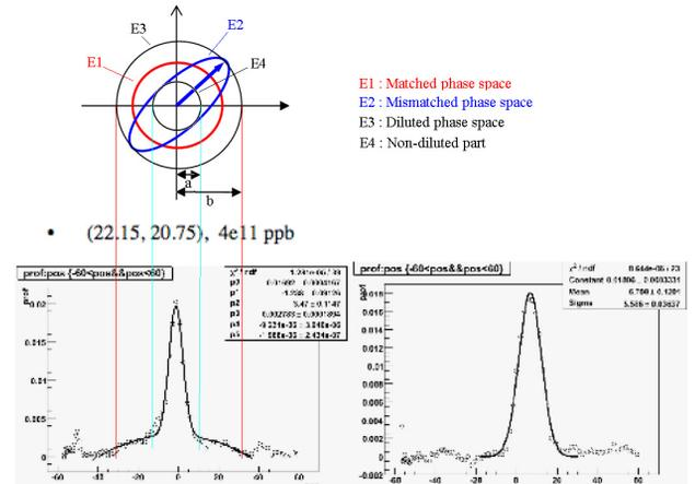
Figure 11: MR beam profiles shows by MR FWPM before (left) and after (right) envelope and its explanation (dilution beam size: b; non-dilution beam size: a; b:a=3).
