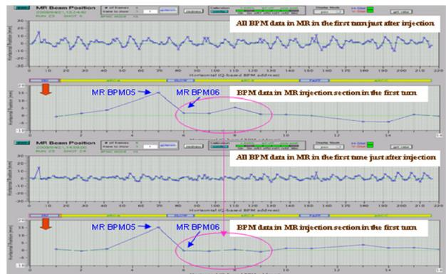
Figure 4: Orbit tuning due to “Without bump scheme”.
