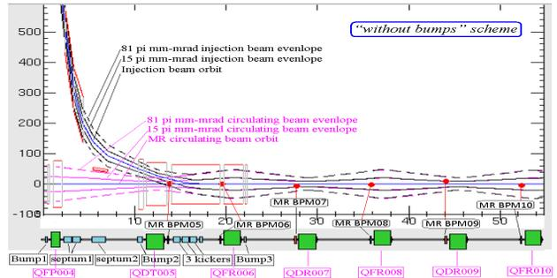
Figure 2: “Without bump scheme” of MR injection.
