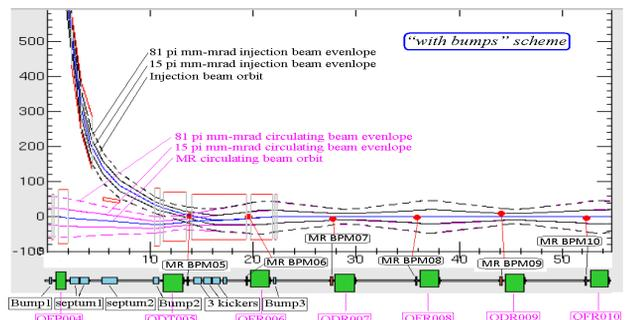
Figure 3: “With bump scheme” of MR injection.
