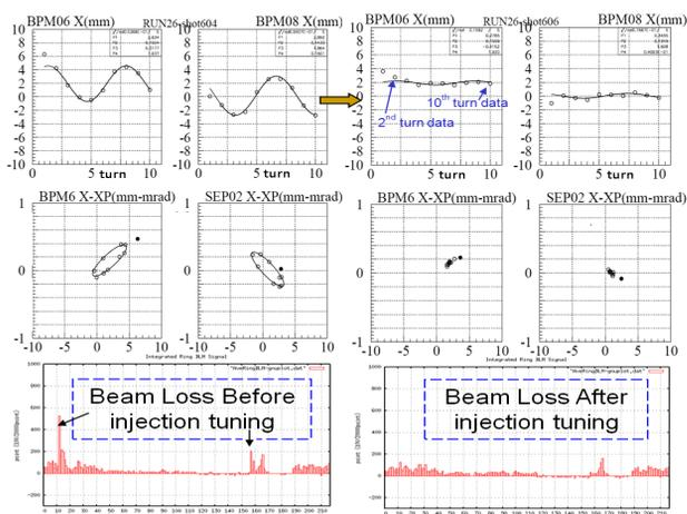
Figure 6: MR injection tuning after MR COD correction (left: before correction; right: after correction).
