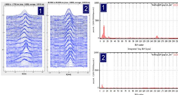
Figure 10: Beam profile mountain views at MR IPM and MR beam loss before and after injection envelope matching (1: mismatched; 2: matched).
