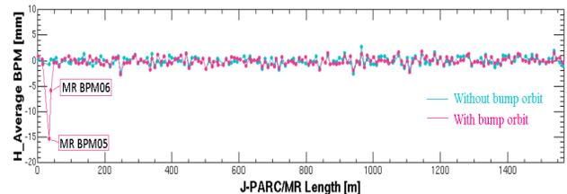
Figure 8: Show of the MR orbit with injection bump.
