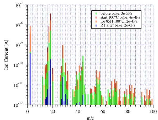
Figure 5. RGA variations before and after baking of the kicker chamber with ferrite cores, before installation to the accelerator tunnel (Oct. 2006).
