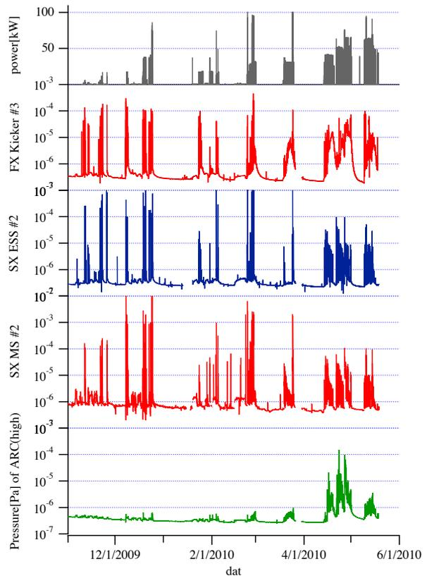
Figure 8. Pressure rise of typical area and beam intensity trend of Nov.2009—May.2010.
