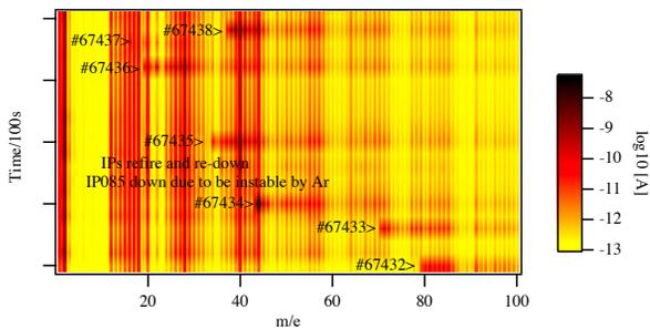
Figure 7. Surface plot of RGA ion current of SX MS#2 at 2/3/2010 19:00 in Fig.6. Scanning time is 1s/au. #xxxxx means shot number.
