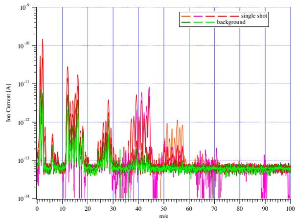
Figure 4. RGA of Kicker#1 with several single shots (2/3/2010). Each pressure rise up about  $2 \times 10^{-5}$  Pa.
