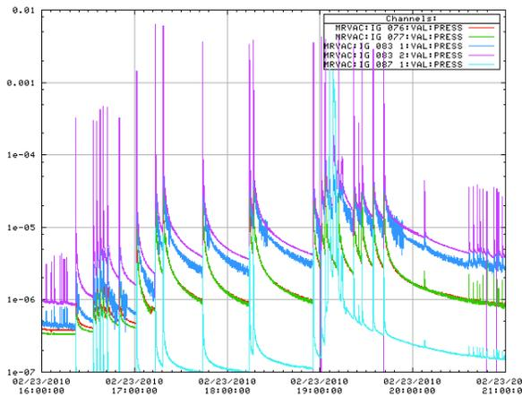
Figure 6. The pressure rise of SX chambers by many 30—70Tppp (100kW) single shots. SX MS#2 is purple line.
