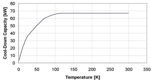
Figure 1: Cooldown capacity of refrigerator.
