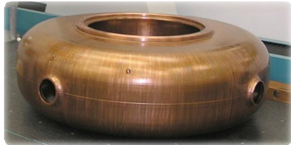
Figure 3: There are four ports on the cavity equator. They are made by extruding: a pilot hole (upper photo) is first cut, followed by pulling a die through the hole. Lower photo shows the finished ports.
