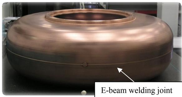
Figure 2: MICE cavity: two half shells are joined by e-beam welding to form the cavity.
