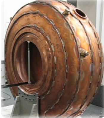
Figure 5: Physical measurements: CMM scan setup of MICE cavity at LBNL.
