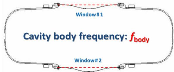
Figure 7: The measured frequency is referred to as cavity body frequency with flat windows as shown. The cavity frequency with curved windows is considered to be a perturbation on the cavity body frequency.
