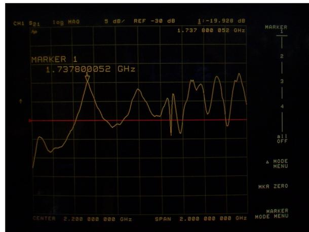
Figure 4: Spectra of the metglas cavity
