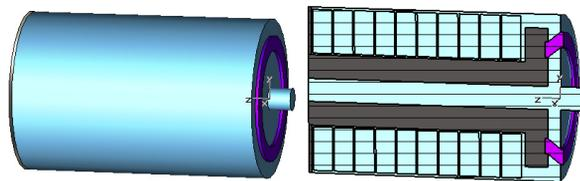
Figure 1: Cavity model of Mini-LIA
