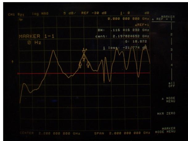
Figure 5: Q-value measurement of TM<sub>120</sub> mode
