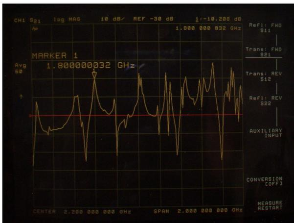
Figure 3: Spectra of the empty cavity
