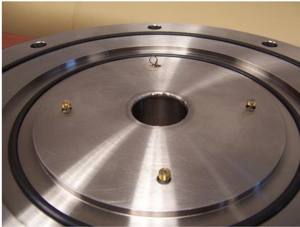
Figure 2: Field probes of Mini-LIA cavity
