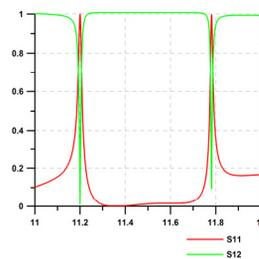
Fig. 3: S-parameters calculated by HFSS.
