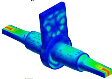
Fig. 5: Spurious resonance example.
