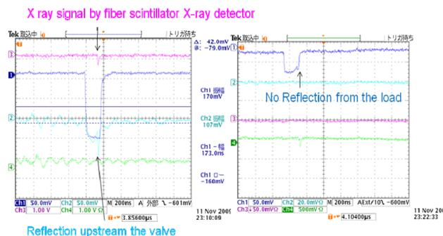
Fig. 9: Waveforms of breakdown events at the valve.
