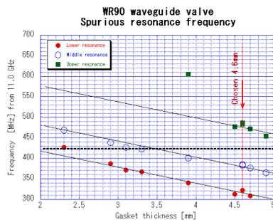
Fig. 6: Spurious resonance frequency vs gasket thickness.
