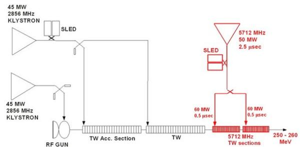
Figure 1: SPARC upgrading with a C-band system.
