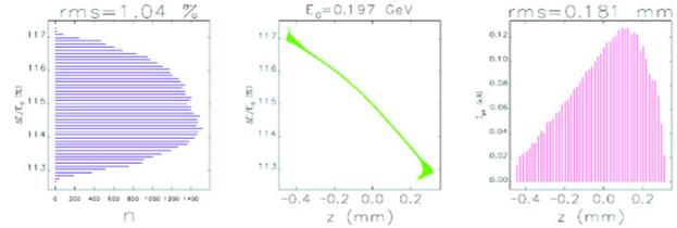
Figure 5: Longitudinal energy and current distribution of the tracked 200 pC electron beam, ( $N_p=50\text{kp}$ ).
