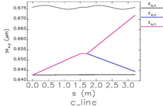
Figure 6: Horizontal emittance dilution as effect of random (blue curve) and cumulating (red curve) accelerating sections misalignment  $\Delta x=500 \mu\text{m}$ .
