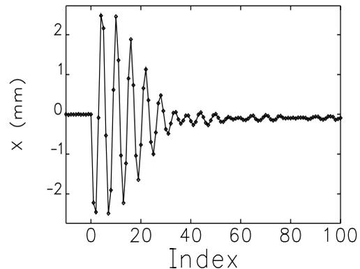
Figure 1: Horizontal betatron motion after injection.
