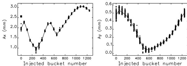
Figure 2: Horizontal (left) and vertical (right) amplitudes of bunch 0 motion as a function of the injected bucket number.
