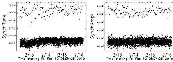
Figure 5: Synchrotron tune (left) and amplitude (right). The points at the top of the plots correspond to injections into bucket 0.
