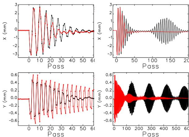
Figure 6: Comparison of the measured and simulated beam motion after injection. Top row is horizontal motion, bottom row is vertical motion. Red line shows measurements and black line shows simulations. Left column presents zoomed-in version of the right column.
