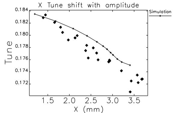
Figure 7: Comparison of the measured (symbols) and simulated (line) horizontal tune shift with amplitude.
