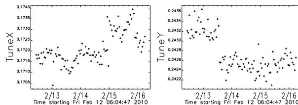
Figure 4: Horizontal (left) and vertical (right) betatron tune variations over the course of five days. Only injection into bucket 0 is shown.
