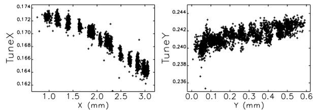
Figure 3: Betatron tune dependence on the oscillation amplitude. Left plot - horizontal tune vs horizontal amplitude; right plot - vertical tune vs vertical amplitude.
