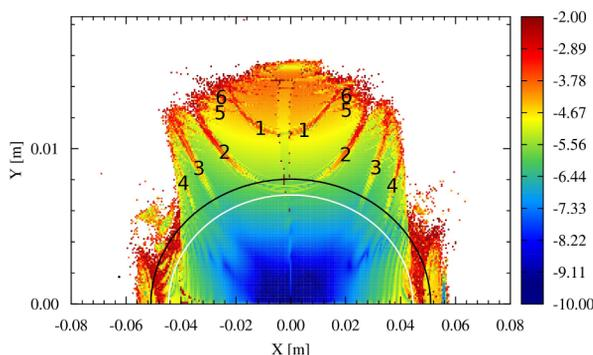
Figure 5: Dynamic aperture for HESR design tunes at  $\gamma_{tr} = 6.2$  including orbit diffusion coefficient on color scale. The smaller the orbit diffusion coefficient the more stable the particle motion is. The most serious resonances are identified from Fig. 4 as 1) (1,7,61); 2) (0,8,61); 3) (1,-9,-61); 4) (2,-10,-61); 5) (5,-8,-23); 6) (4,-7,-23)
