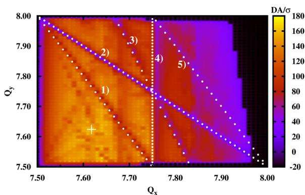
Figure 3: Tune scan for  $\gamma_{tr} = 6.2$  and on-momentum particles tracked over 1000 turns. The dynamic aperture in terms of beam size  $DA/\sigma$  is plotted in color scale against the transverse tunes  $Q_x$  and  $Q_y$ . The value of -20 is artificially introduced to differentiate unstable linear lattice (-20) from zero dynamic aperture. The design tunes are marked with a white cross. Enumeration of resonances is explained in text.
