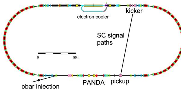
Figure 1: HESR lattice: Upper straight is housing electron cooler and stochastic kickers, lower straight contains injection, PANDA experiment with target, and stochastic pickups. The second dipole from each end of both arcs is missing for dispersion suppression in the straight sections and  $\gamma_{tr}$  adjustment.
