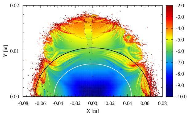
Figure 6: Dynamic aperture for HESR design tunes at  $\gamma_{tr} = 6.2$  including orbit diffusion coefficient on color scale. The smaller the orbit diffusion coefficient the more stable the particle motion is.
