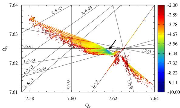
Figure 4: Frequency map for HESR design tunes at  $\gamma_{tr} = 6.2$  calculated from first and second thousand turns. The identified resonances are marked by lines and the corresponding resonance condition (m,n,p). Design tunes are located at the blue spot marked by the arrow.
