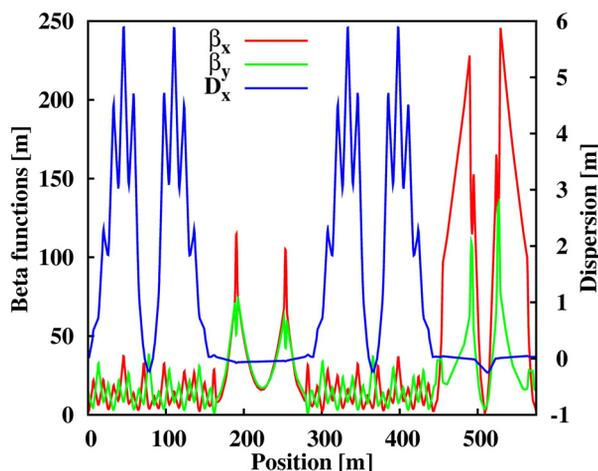
Figure 2: HESR optics for  $\gamma_{tr} = 6.2$ : electron cooler is located at roughly 220 m, the PANDA target at 509 m. The straight sections are nearly dispersion-free except for around the PANDA target where a kink is introduced by the PANDA chicane dipole magnets.
