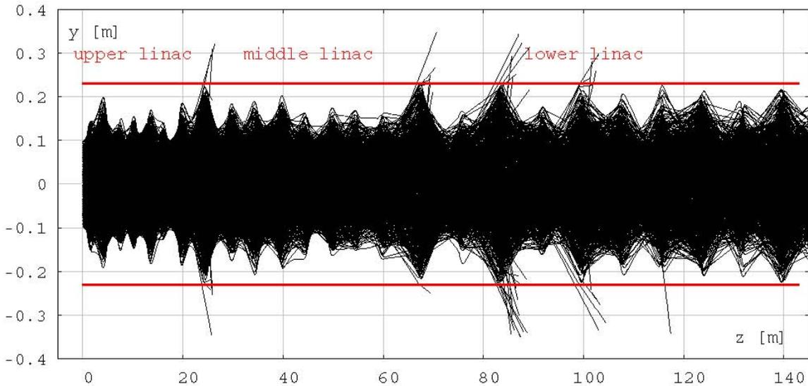
Figure 7: Vertical projection of the muon trajectories along the linac confined within the vacuum chamber walls.
