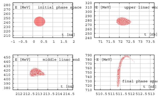
Figure 5: Longitudinal phase space at four points along the linac.
