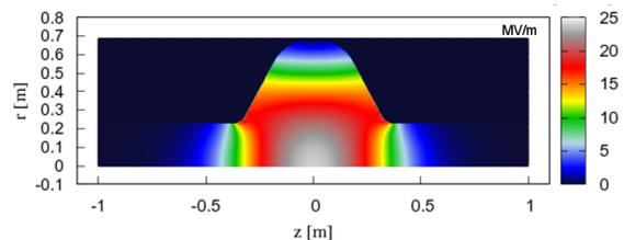
Figure 2: Total electric field for the  $\beta = 1$  RF cell.
