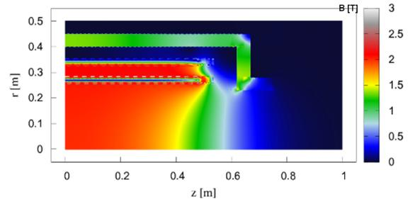
Figure 1: Total magnetic field of the shielded solenoid for a peak value of 2T with the current densities of 165.75 and  $-82.87 \text{ A/mm}^2$  for the inner and outer coil respectively.
