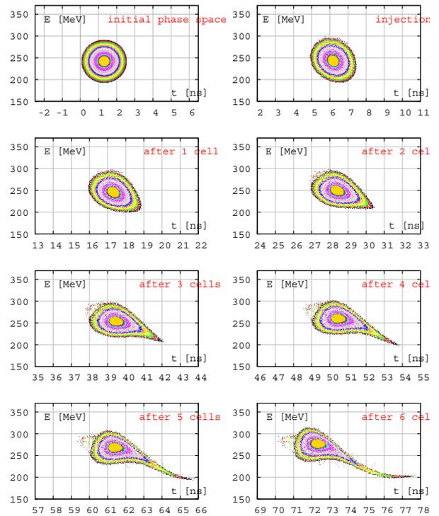
Figure 4: Filamentation of the longitudinal phase space.
