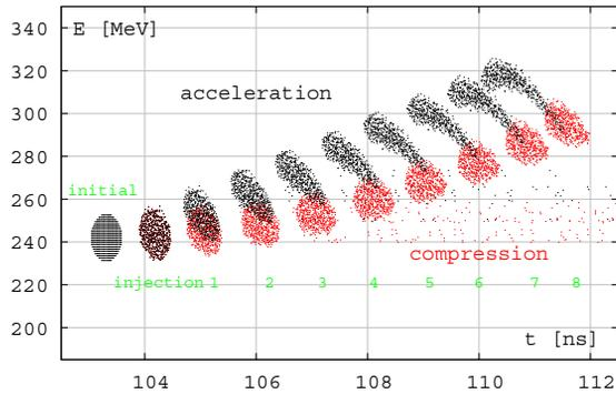
Figure 3: Two choices for the RF phases depending whether acceleration or longitudinal phase space compression is desired.
