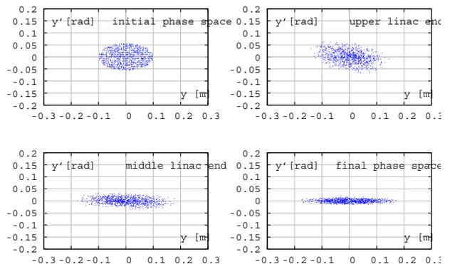
Figure 6: Vertical phase space at four points along the linac
