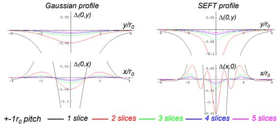
Figure 3: Comparison of the gradients from smooth and sliced beams
