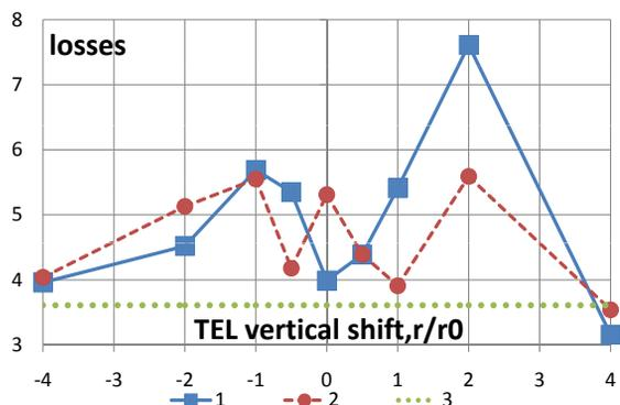
Figure 5: Results of the first set of simulations. Vertical scale is increased by a factor of  $10^4$ , losses normalized by initial beam intensity. "1" corresponds to  $\xi_{TEL} = 0.006$ , "2" corresponds to  $\xi_{TEL} = 0.003$ , "3" corresponds to TEL turned off.
