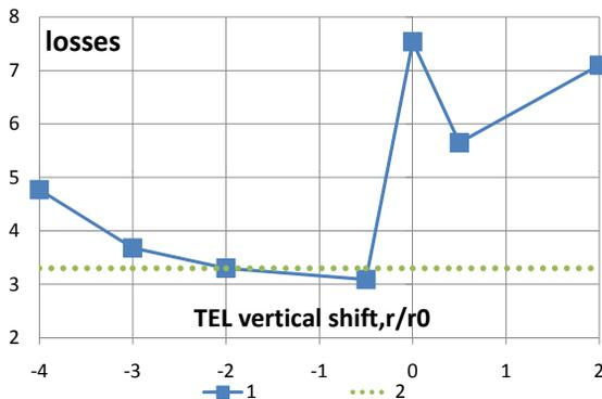
Figure 6: Results of the second set of simulations. Vertical scale is increased by a factor of  $10^4$ , losses normalized to initial beam intensity. "1" corresponds to  $\xi_{TEL} = 0.003$ , "2" corresponds to TEL turned off.
