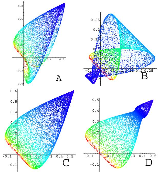
Figure 4: Footprint distortions, initial tunespread generated by a Gaussian beam of equal size. A - Gaussian EL,  $\xi_e = 0.5\xi_p$  with  $1r_e$  shift; B - SEFT,  $\xi_e = \xi_p$ , no shift; C - Gaussian EL,  $\xi_e = 0.5\xi_p$  with  $\pm 1r_e$  tilt; D - SEFT,  $\xi_e = 0.5\xi_p$ , no shift.
