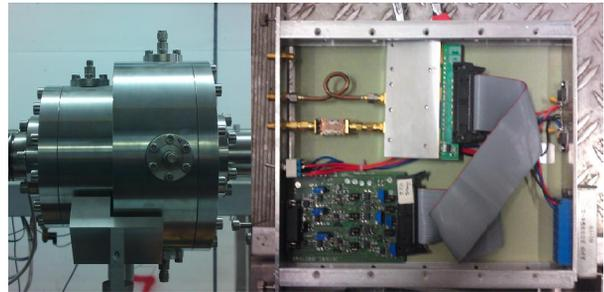
Figure 5: rf monitor (left) and rf board (right) used for the measurement.
