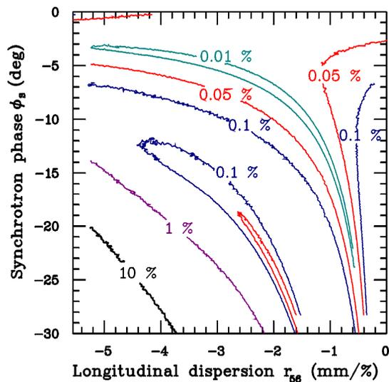
Figure 3: Hill plot of the expected energy spread ( $\Delta E_{RMS}/E$ ) as a function of the longitudinal dispersion  $D_L$  and the synchrotron phase  $\Phi_S$ .
