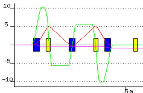
Figure 4: Lattice of the first recirculation bend, the longitudinal dispersion  $D_L$  is plotted in purple (unit mm/%), dipoles blue and quadrupoles yellow.
