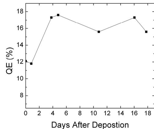
Figure 2: Cesium Telluride quantum efficiency: (a) time evolution during Cesium in the fabrication chamber. The curves correspond to three depositions made at different rates; (b) lifetime of photocathode kept in preparation chamber for eighteen days. The quantum efficiency can show a slight increase in the initial few days, but typically it will start decreasing after a few weeks.
