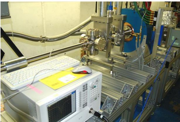
Figure 1: The new AWA RF gun (behind the blue solenoid) will replace the present drive gun. The two gate valves, and the long actuator connected to the back side of the gun, allow the insertion of the Cesium Telluride photocathode without exposing it to air.
